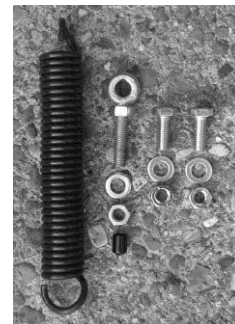
Spring, (depends on purchase) Eye bolt, 2 x nuts, washer, cap 2 x mounting bolts, nuts, washers
